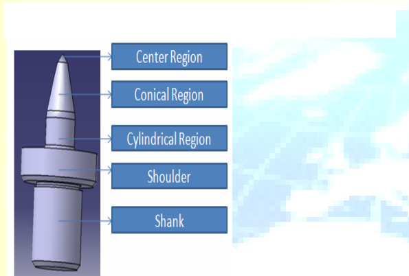
FIGURE:5 Conical sections in order to provide the primary contact area to reduce tool wear [1]
